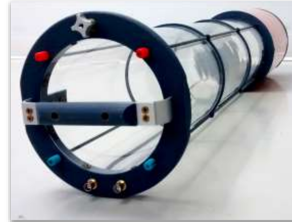
Transmit/Receive “birdcage” coil for 7T Agilent Application: Rabbit heart Collaboration: Dr. Lesage (Montreal Heart Institute)
