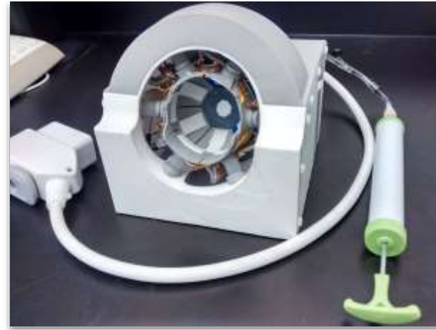
13-channel adjustable coil for 3T GE Application: Neonatal human brain Collaboration: Dr. Lodyginsky (Ste-Justine Hospital)
