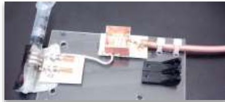
Transmit/Receive “solenoid” coils for 7T Application: Ex vivo tissue Collaboration: Dr. Stikov (Polytechnique)
